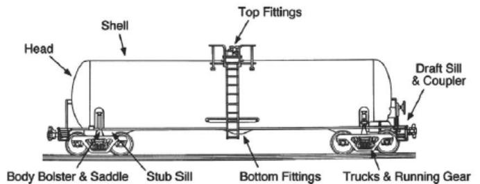
The tank is made of steel plate, 7/16 of an inch thick. An oil tank car is typically loaded from the top valve and unloaded from the bottom valve. Loading or unloading each car may take several hours, but multiple cars in a train can be loaded or unloaded simultaneously.
