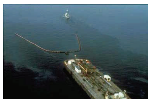
Oil containment boom allows water to pass below the boom skirt while stopping the oil floating on the water.
